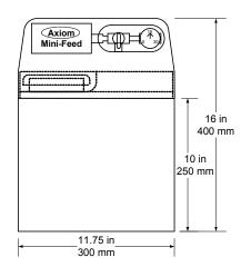
Depth - 11.75 in 300 mm Clearances – Right Side and Top - 12 in 305 mm Weight When Full 60 lbs/27 kg. Discharge 1/2" FPT
