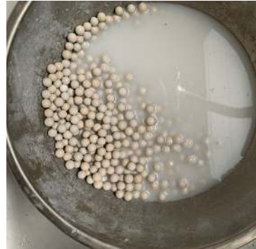
Figure 8: Neutralization media that has been rinsed with clean water
