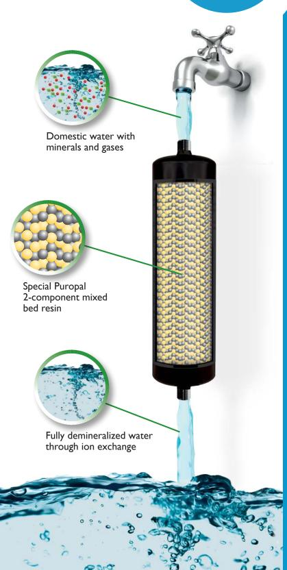
Demineralizers prevent valuable metal components in closed loop hydronic systems from corroding and scaling
