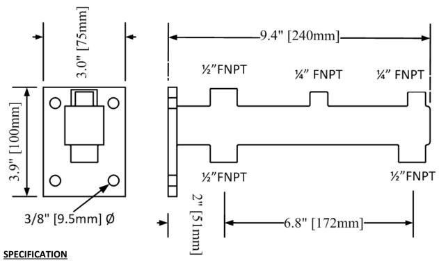
Expansion Tank Bracket shall be AXIOM INDUSTRIES LTD. Model HN-1. Bracket shall be constructed out of welded steel material and shall include: quantity three ½" FNPT connections; and quantity two ¼" FNPT connections. Unit shall be mounted on a wall using lag bolts connected to an appropriate material/structure designed to support the weight of the bracket, expansion tank, and any related system piping material.
