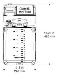
Depth – 11.0 in (280 mm) Clearances – Right/Left - 0 in (0mm) provided side screws on lid are removed upon installation Clearances – Top – 3" (75mm) Weight When Full 50lbs (23kg) Discharge ½" FNPT
