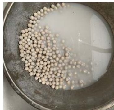
Figure 5: Neutralization media that has been rinsed with clean water
