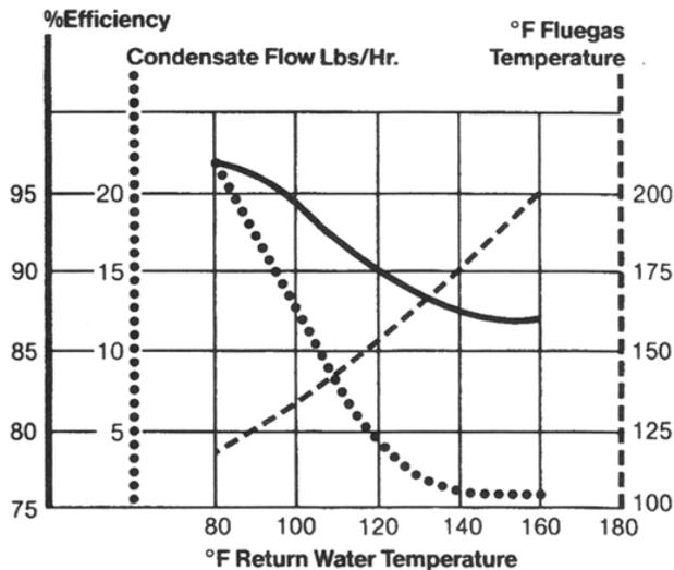
It's the same with condensing boilers that advertise efficiencies as high as 98%. The reality, illustrated by the chart\* to the left, is that those numbers are only achievable if the boiler return water is  $\approx 80^\circ\text{F}$  ( $27^\circ\text{C}$ ). The boiler **will not condense at all** if the return water is **at  $\approx 130^\circ\text{F}$  ( $54^\circ\text{C}$ ) or higher**, in which case it's an expensive mid-efficient boiler.
