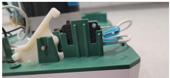
Figure 3 High Level Safety Switch on AP43-HTS in N.O. position
