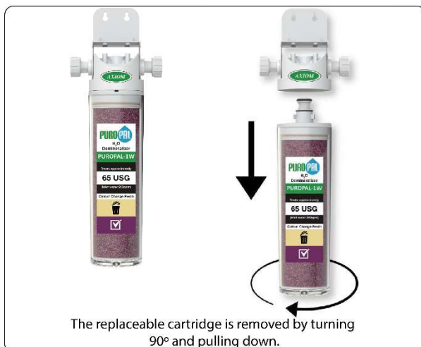
Figure 2 - Replacing cartridge
